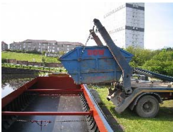
Figure 5.3 Skip loading into a vessel
